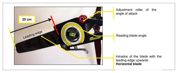
Horizontal blade, leading edge upward, place the adjustment tool at 25 cm from the tip of the blade, intrados side (flat), handle down.
