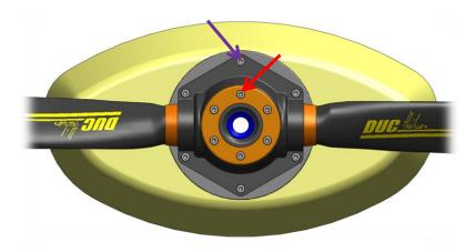
Slightly untighten the **propeller fixing screws** and the **hub assembly screw**.
