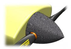
After a final verification (position and orientation of parts, tightening...), mount the spinner on its plate **by tightening the spinner screws to a torque of 4Nm (0.4kg/m)** with the appropriate tools.
