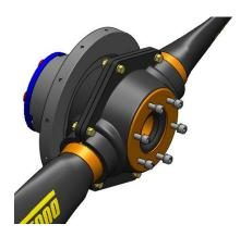
At this point, the propeller is installed on your aircraft with the spinner mounting plate.
