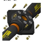
From the front hub, set up the 6 screws and washers for hub assembly.
