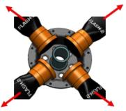
If specified on the propeller's Delivery Note, respect the order of placement of the blades in the hub.
