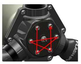
Gradually tighten in 2 or 3 times the 6 CHC M8 propeller fixing screws at 20 Nm.
