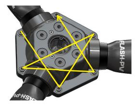
Now, make a **progressive tightening in cross** in 2 or 3 times to reach the **tightening torque 25 N.m**.
