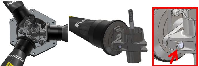
While keeping the satellite laid on the back half-hub, slot the FLASHBLACK/-2 & SWIRLBLACK-3 blades one after the others into the satellite groove and into the back half-hub.
