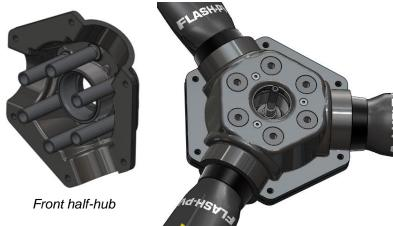
Ensure the good introduction of the blades in their place. Place the front half-hub. This one must include 6 carbon tightening recovery columns. Watch if the parts are aligned for the assembly.
