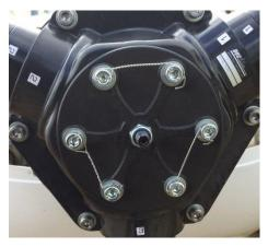
10) After a final check (position and orientation of parts, tightening, ...), install the spinner on the spinner mounting plate by **tightening the screws to a torque of 4 Nm (0.4kg / m)** with the appropriate tools.
