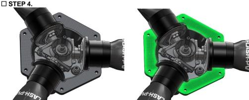
Place the 2 (2-blade) or 3 (3-blade) carbon **foils** on the flat of the back half-hub. **Be careful with the manipulation, fragile parts.**
