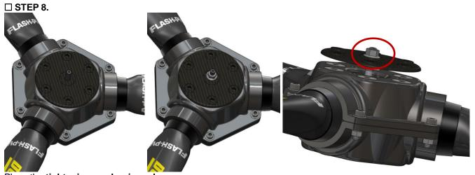
Place the **tightening washer in carbon**. Put the safety return spring in compression by pushing the carbon washer and screw the **NyIstop nut M10 at the beginning of this one and keep this position for the M10 nut until the setting of the propeller**.
