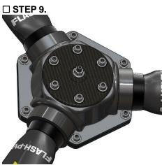
Put the 6 Fixation screws CHC M8 + Washer in the fixations drillings of the propeller.
