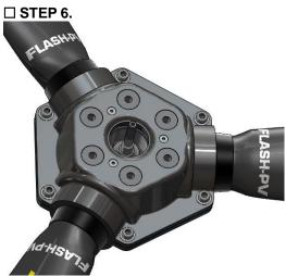
Place the Screws CHC M8x30 + Washer over the top and the Nylstop nut behind for the assembly of the 2 halfhubs.
